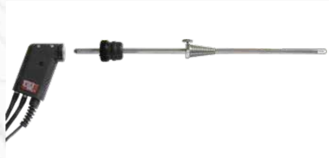
Gas sampling probe for industrial combustions, unheated, without filter for short, complete emission monitoring including NO 2 /SO 2 , probe handle for exchangeable tubes, with 9 foot gas sampling line (VITON)
