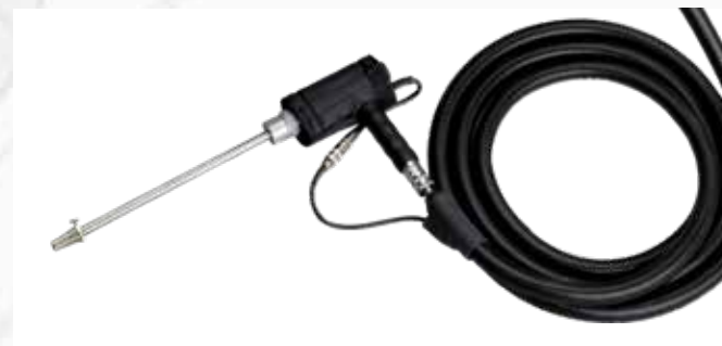
Gas sampling probe for industrial combustions, with heated probe handle and easily replaceable quartz glass wool filter for exchangeable tubes
