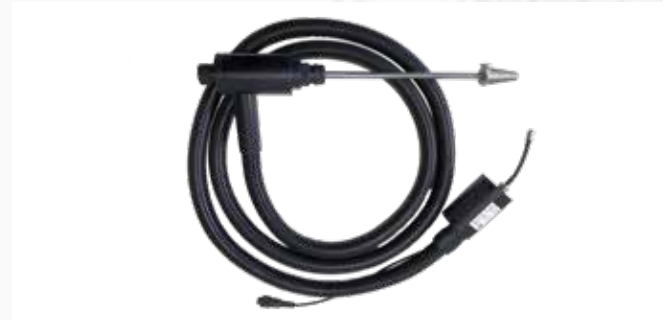
Heated gas sampling probe with heated sampling line, length 9 foot, 266°F temperature regulated Gas temperature measurement using K-type thermocouple. With heated, easy replaceable quartz wool filter.
