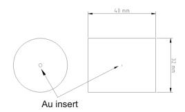
Schematic drawing of the phantom
